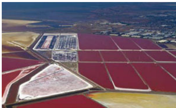
Cargill's evaporation ponds concentrate salt and algae. Courtesy of Cargill
